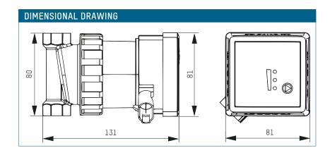
TacoFlow2 PURE PLUS | DHW circulation pumps for potable water systems High-efficiency DHW circulation pump in glandless design with brass housing, insulation shell and plug connection.
