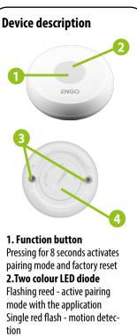
3. Flood Sensors 4. Battery socket
