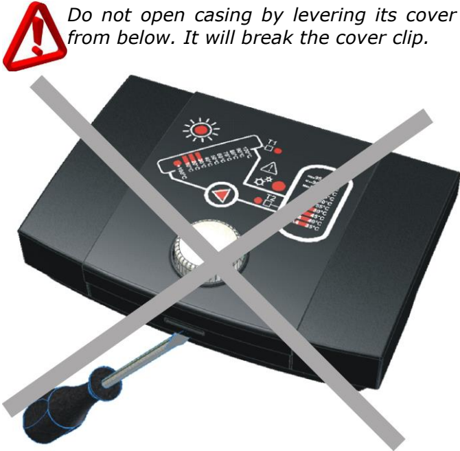
Fig. 11.2 Incorrect method of casing opening
