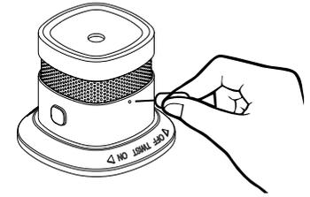
To set the device into pairing mode, press and hold the network button for 3 seconds.
