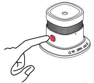
To test or to mute the alarm, press and hold the Test / Mute Button for 3 seconds.
